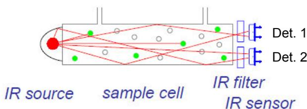
fig. 1 Example set-up with dual channel sensor
